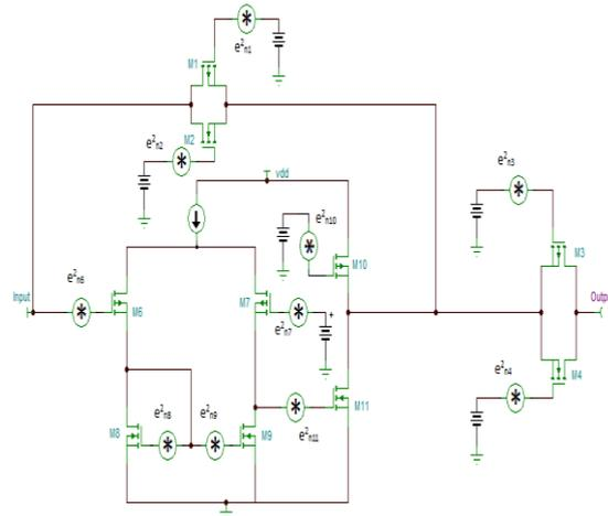
Figure 2.The noise model for circuit diagram in figure 1.
