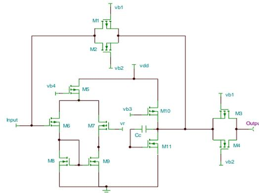
Figure1. CMOS current mode preamplifier circuit
